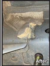
8. Clean excess caulk from the outside of the frame to allow for receiver hitch installation.
