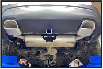
10. Reinstall the exhaust and exhaust pipe clamp. Do not reinstall exhaust side brackets at this time. Continue to support exhaust using a jack or stand.
