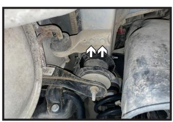
Fully support exhaust using jack(s) or stand(s). Using a 13MM socket with 5" extension, remove the two (2) bolts from the exhaust bracket. Do this on both sides of the vehicle.
