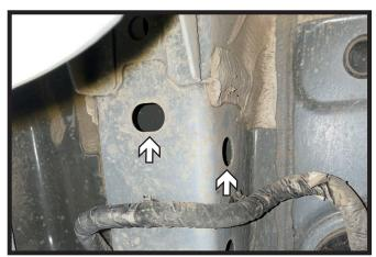
3. **Trailhawk Models**: Using a 21MM socket, remove the two (2) bolts from the frame. Do this on both sides of the vehicle.
