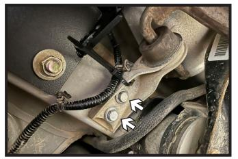
12. Reinstall the exhaust brackets on each side of the vehicle.
