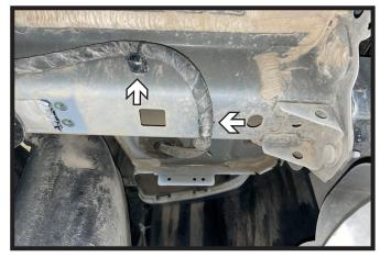
If wire loom is present on the passenger side of the vehicle, unfasten clips holding the loom to the frame. Let wire hand below the frame rail.
