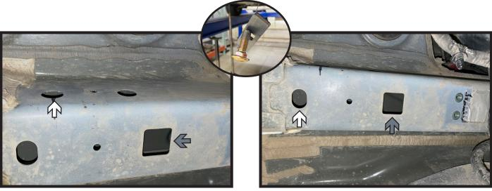
5. Run the lead wire from rear hole (white) on the side of the frame to the access hole (gray). Place spacer plate onto wire, then attach lead wire to the end of a 1/2" carriage bolt (inset). Pull bolt and spacer plate through the frame but do not pull bolt through the hole.
