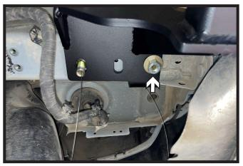
9. Trim down the lead wires to roughly 10". Hold wire loom out of the way and raise the receiver hitch into place. Pull lead wires through the corresponding holes. Remove lead wire from the rear bolt and loosely install conical washer and hex nut using a 3/4" socket with 10" extension. Ensure the teeth of the conical washers are towards the hitch.
