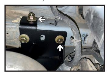
11. Remove lead wires from the remaining two (2) bolts and loosely install conical washers and hex nuts. Ensure the teeth of the conical washers are towards the hitch. Do this on both sides of the vehicle. Tighten all bolts at this time.
