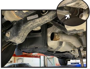
2. Using a 15MM socket with ratchet, loosen the one (1) nut (inset) from the exhaust clamp. Push exhaust toward the front of the vehicle and remove. Set aside the exhaust to be reinstalled later.
